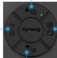
Short press to switch the IR illuminator brightness
